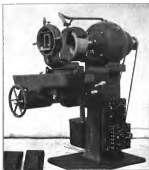
Fig. 4938. Motor-Driven Universal Tool Grinder. Gisholt Machine Co.
